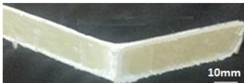
Figure 9. The mode of failure by impact of chopped-GFRP
