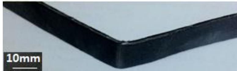
Figure 10. The mode of failure by impact of Toyota's bumper material
