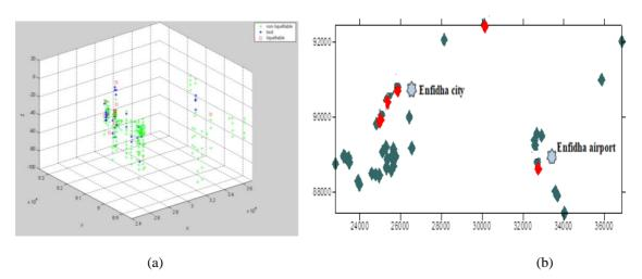
**Fig. 3:** liquefaction risk based on level A identification: (a) georeferenced 3D diagram; (b) Sample location (Sites with a confirmed risk of Level A liquefaction are shown in red)
