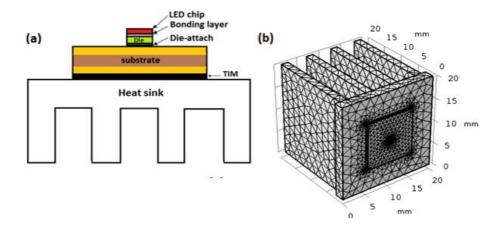
Fig. 1: (a) The structure of the LED package (b) Dimensions of the heat sink
