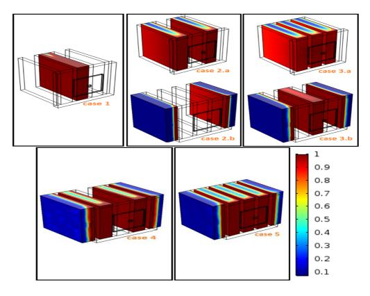
Fig. 4: Liquid PCM volume fraction distribution at t = 5000s
