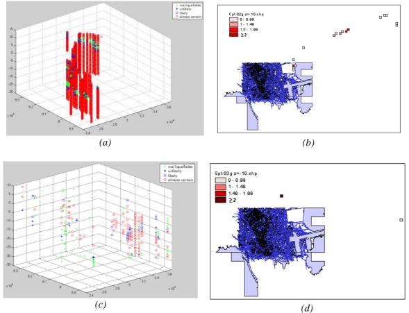
**Fig. 4:** Risk of liquefaction estimated according to the CPT and SPT test: (a) Risk according to the CPT test spatially in 3D; (b) Risk according to the CPT test at depth z = -10m; (c) Risk according to the SPT test spatially in 3D; (d) Risk according to the SPT test at depth z = -10m;
